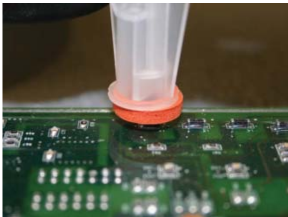
Localized extraction system seals over specific components.
